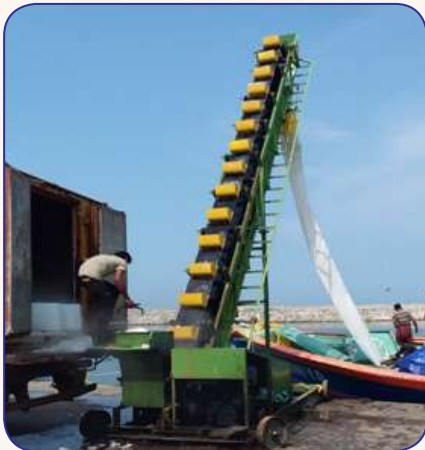
Ice loaded in boats using conveyor at Colachel Fishing harbour
