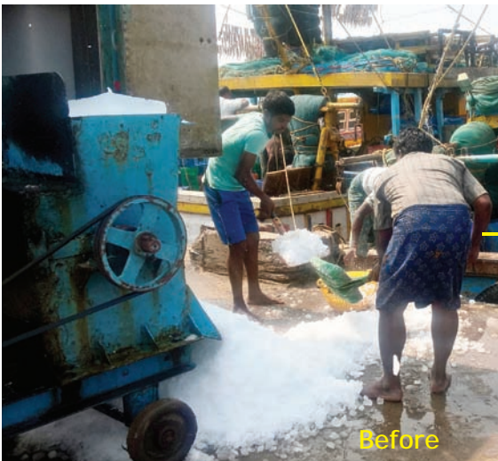
Improved ice handling at Kakinada harbour by providing a stainless steel extension tray to the ice crusher and transferring the crushed ice directly in to fishing vessel, avoiding contact with floor
