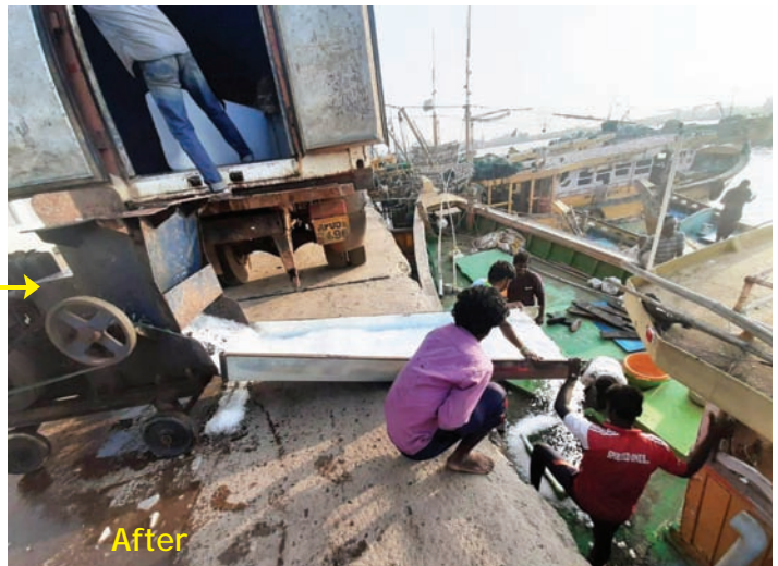
Improved ice handling at Kakinada harbour by providing a stainless steel extension tray to the ice crusher and transferring the crushed ice directly in to fishing vessel, avoiding contact with floor
