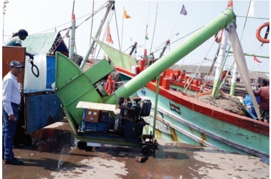
Transferring ice block directly from vehicle to ice crusher and then the crushed ice directly in to the fishing boat at Veraval harbour
